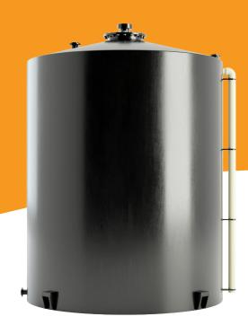
NIPLAST® chemical storage tanks are constructed from the highest rated welding technique within that design code, ie. the butt fusion of extruded thermoplastic plates. High precision automated but fusion machine welds ensure tank integrity over design lives of 20 years. Third party employee certification to EN 13067 by The Welding Institute (TWI) underwrites that tank integrity.
